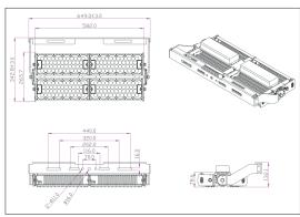
**LEDX PHOENIX GROW** 480 watts including power adapter and power adapter box
